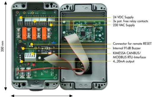
KIMESSA CANBUS/ MODBUS RTU-Interface
